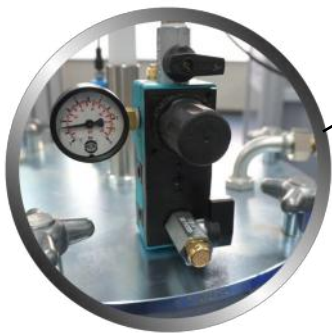
Pneumatic unit compressed air supply with ventilation for pressure container
